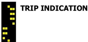
The states of the 7 trips are indicated by 7 bars, the top most being trip 1, the bottom one being trip 7. For example, the figure indicates that trips 1, 2 and 3 are on, trip 4 is overridden, trips 5 and 6 are off and trip7 is inhibited.
