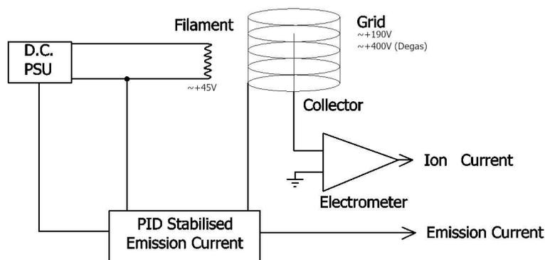
The measurement process is shown in the schematic. In the PVCs, the filament is heated by a high stability, low noise, constant current source. The emission current from the filament to the grid is PID stabilized at the desired value. The controller simultaneously measures the ion current **AND** the emission current to determine the pressure.
