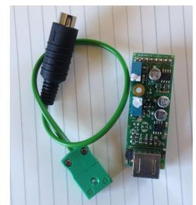
The 'K' module has a 4 pin mini-DIN connector - see below. To assist with installation, it can be provided with a 150mm long mini-DIN to mini-thermocouple adaptor cable, as shown in the photograph.
