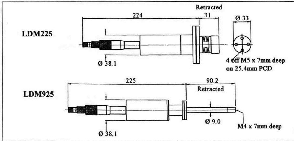
Figure 5. LDM225 and LDM925 Micrometer Linear Motion Drives.
