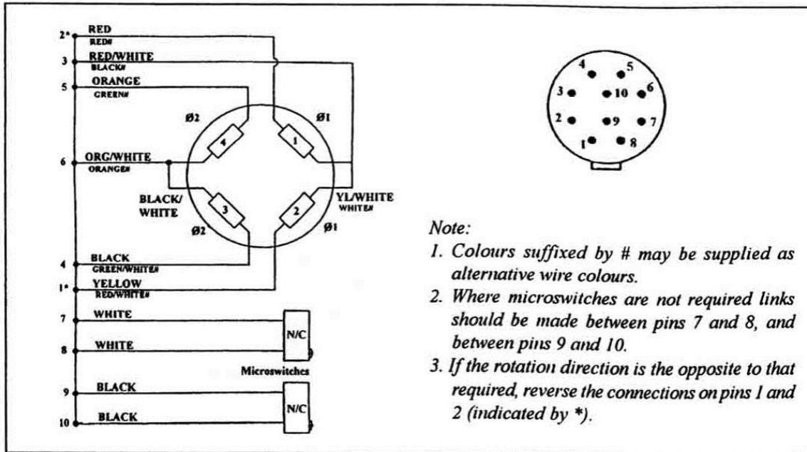
Figure 14 - Series Wiring Diagram
