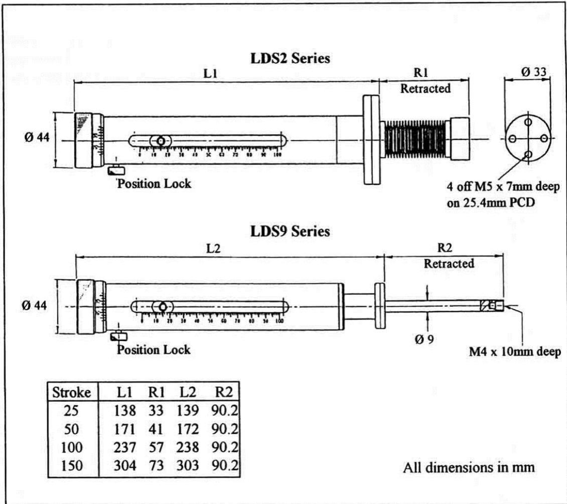
Figure 1- LDS2 and LDS9 Series Linear Motion Drives
