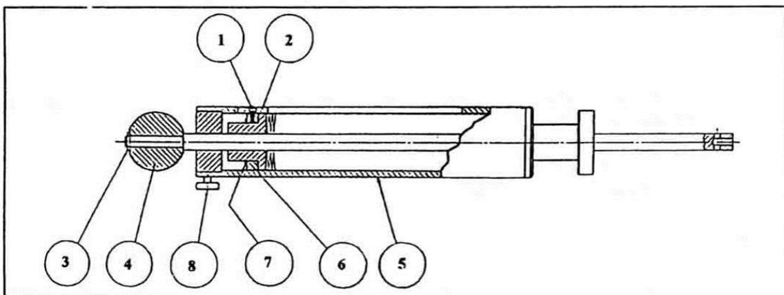
Figure 4 - Components of the LDP9 Drive Mechanism
