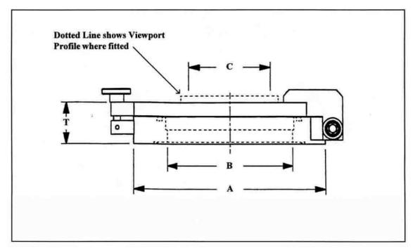
Figure 1- Dimensions of the HD and HD..V loadlock doors
