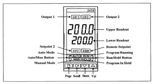
Figure 2 - Front panel controls and displays of the 2408 temperature controller
