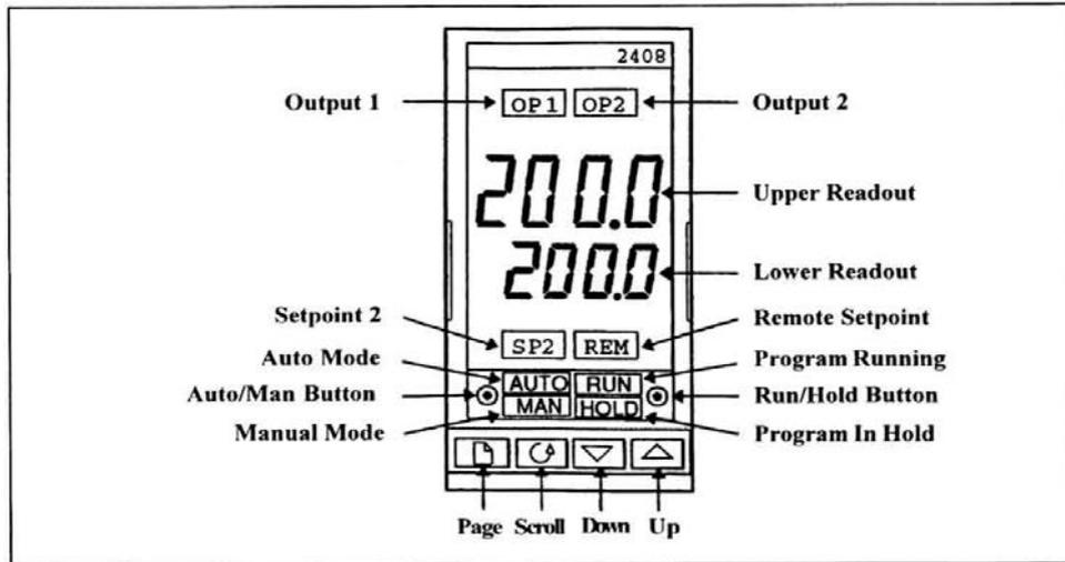
**Figure 2 - Front panel controls and displays of the 2408 temperature controller**
