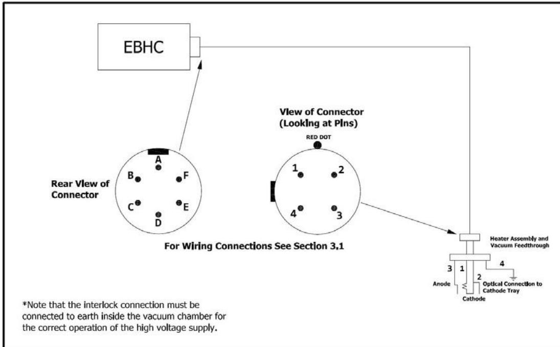
**Figure 1 - Power cable connections between the EBHC and the heater module**
