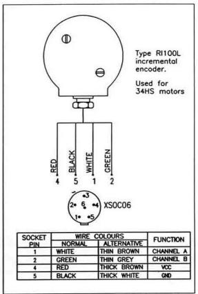
Wiring diagrams for incremental motor encoders
