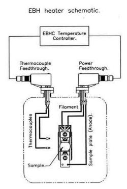
**WARNING**: It is very dangerous to leave feedthrough contacts isolated, especially during bakeout and when high voltages are present near to the sample. It is the responsibility of the user to be aware of electrostatic charge buildup and to provide suitable earthing.
