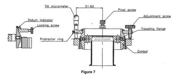
A datum indicator attached to the gimbal may be aligned with either the X or Y micrometer axis, whichever is regarded as the zero datum. Any plane of rotation, relative to the zero axis datum, may be selected by rotating the protractor ring to the required angle.
