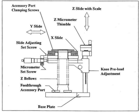
Figure 3 - Cross-section through the LCM translator
