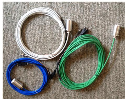
*Ion gauge cables bakeable to 200°C*
