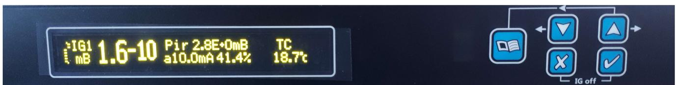
The picture shows one of many ways in which the values of the gauges and thermocouple are displayed for both the PVCuni and PVCduo. For more information, please refer section 4.
