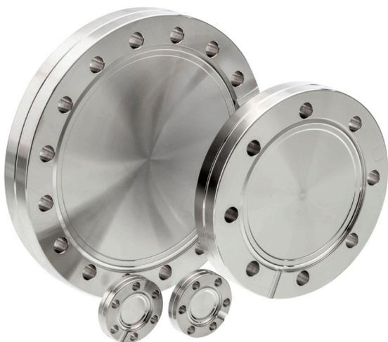
Fixed blank flanges are available in the full range of sizes as indicated in the chart below. They are normally used to blank off unused chamber ports to create a leak-tight assembly. It is also possible to machine them as required for the fixing of special tube sizes or components that are not covered by the standard range of sizes.
