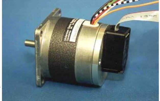
Where customers require an encoder for use with control systems not supplied by Mclennan and which require alternative line-counts, the model 'RI' encoder is available with any line count required up to a maximum value of 2,000 ppr. resulting in a measuring resolution of 8,000 steps/rev.
