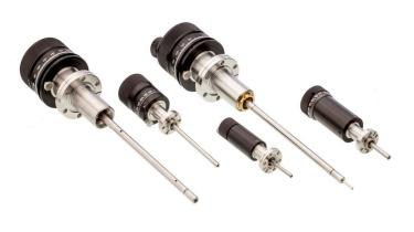
The RD1 is a low backlash, high precision edge welded bellows drive providing continuous primary rotation to a 9.52 mm diameter shaft.
