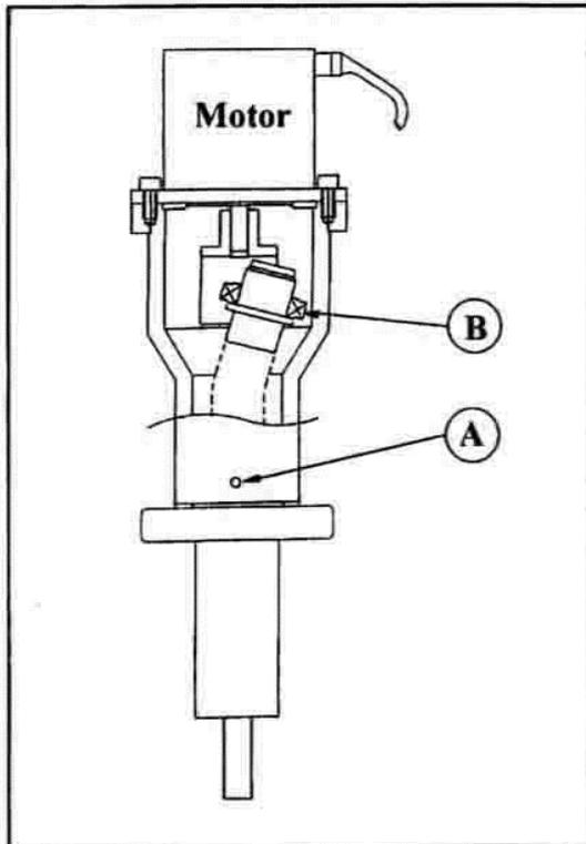
**Figure 8: Direct motor drive
