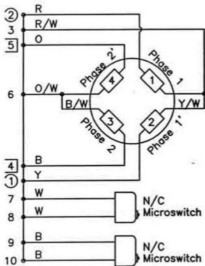
Parallel Motor Wiring
