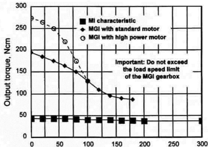
Figure 5 - RD6 and RD7 speed-torque performance
