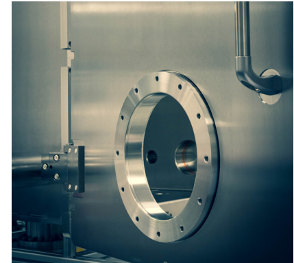
PLD Box Chamber
